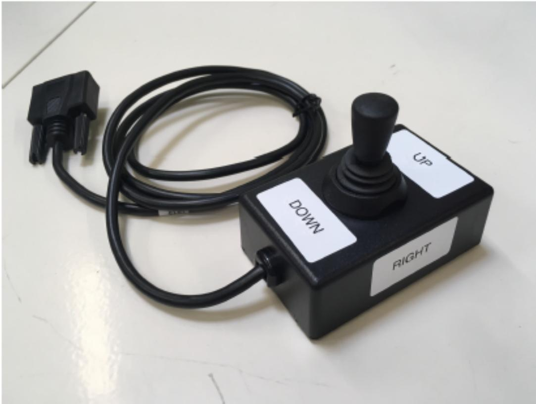
Figure 3-3: Four-way joystick controller
